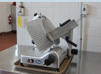
This slicer is extremely sharp and is used for slicing meats and some vegetables to an exact thickness.
