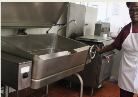
This "tilt skillet" is used for cooking meats and vegetables. It can tilt to allow for draining water or grease.
