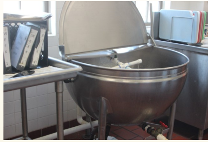
This "thaw pot" uses cold, running water for thawing frozen foods prior to cooking, according to food safety.
