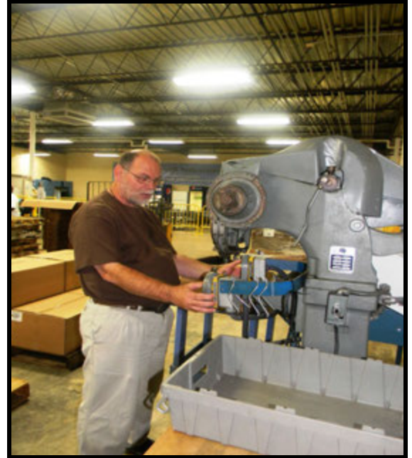
John hard at work operating the riveting machine
